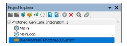
Example: The device ID is *DVA-048*. The **DEVICEID** field in the AVS needs to contain the whole *PhotoneoTL\_DEV\_* prefix and the device ID - in this case, *PhotoneoTL\_DEV\_DVA-048*
