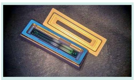
**Emberion's** infrared detector technology and 2018 product introduction focused on a VIS-SWIR (400-1,800nm) linear array solution intended for spectroscopy applications. In 2020, the linear array product will be market ready, and engineering samples of a VIS-SWIR VGA imager product will be launched.
