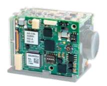
high-definition, real-time video transmission across long cable lengths and multiple slip rings. Ideal for pipeline inspection, surveillance and industrial vision in general, Harrier 3G-SDI boards offer an interface solution supporting HD-VLC technology. These boards fit on compact autofocus zoom cameras. Active Silicon will also launch USB and IP interface boards in the coming months.
