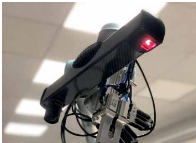
Photoneo's MotionCam-3D camera can inspect objects moving at 40m/s
