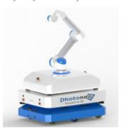
the safety class SIL2 PL.d Category 3. It checks its surrounding environment 33 times per second and the system is able to detect obstacles every 30 ms with a minimum width of 30 mm. It also enables adaptive safety zones. The laser scanner prevents collisions
